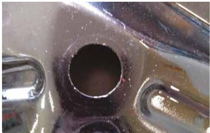
**EN** 10. Reuse the rubber stop from the OEM bonnet following the applicable steps for your Clio IV R.S. depending on it being a first or second generation:
